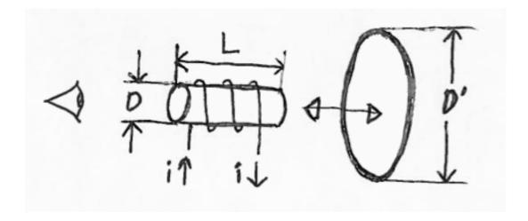
The solenoid has length L and radius R. The solenoid wire has N turns and constant current I flowing clockwise when viewed from the left. The conducting loop has radius R' > R.
