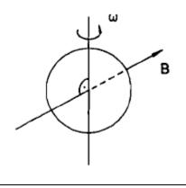
A circular ring with radius, R, rotates with a constant angular frequency,  $\omega$ , about its diameter (see Figure). A homogeneous magnetic induction, **B**, is oriented perpendicular to the rotation axis of the ring.
