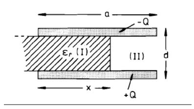
A capacitor (area  $F=a \cdot b$ , separation *d*) is partially filled with some dielectric material with a dielectric constant  $\varepsilon_r > 1$  (see figure). The remaining space between the capacitor plates is empty. The bottom plate carries a charge *Q* and the top plate carries a charge -Q. Any stray fields can be neglected.
